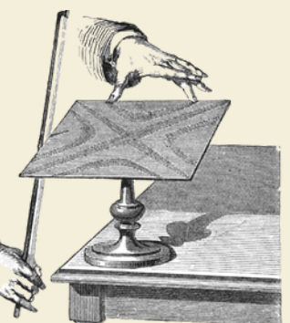
Chladni plate illustration, 1879
